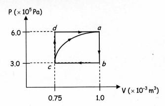
A cylinder with a movable piston contains 0.1 mole of a monatomic ideal gas. The gas, initially at state a, can be taken through either of two cycles, abca or abcda, as shown on the PV diagram above. The following information is known about this system
